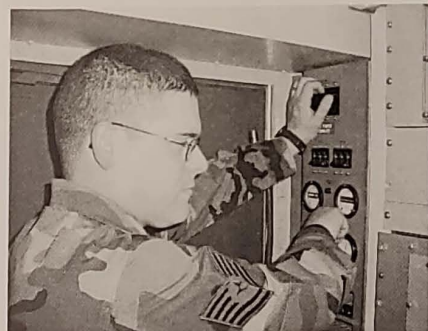
Tech. Sgt. Michael Meek checks the frequency of the incoming voltage on the TRC-170.
